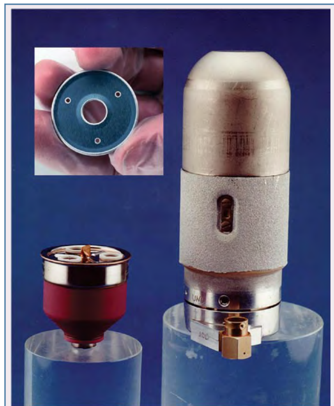
Neutron generator (right) and neutron tube (left), with 1.25-in.-diameter target (inset). All nuclear weapons systems in the US stockpile contain neutron generators that supply a burst of neutrons to ensure initiation of the fission reaction. The units contain tritium and because tritium decays over time, the neutron generators must be replaced periodically.
