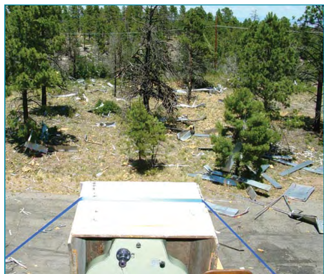
Blowout panels and other debris are scattered up to 300 ft away from building 340 after a 25-lb test shot.
