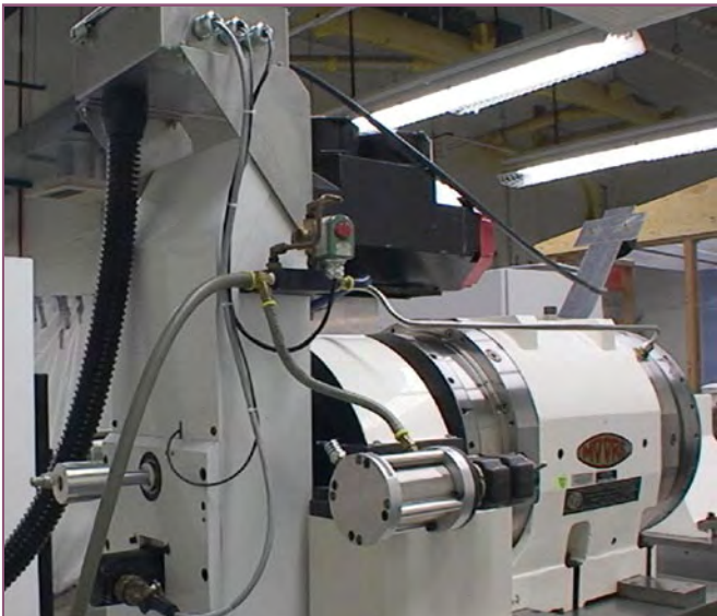
Spindle assembly (rear view). The Moore T-base lathe originally was configured with a hollow-shaft spindle motor through which the vacuum source for holding the part passed to the face of an air-bearing spindle. With this spindle motor configuration no longer available as a stock item, MSM engineers designed a new spindle drive package to accommodate the use of an off-the-shelf spindle motor. The design included equipment required for C-axis (spindle positioning) capability, which in turn enabled the installation of curvic couplings and a part probing system.
