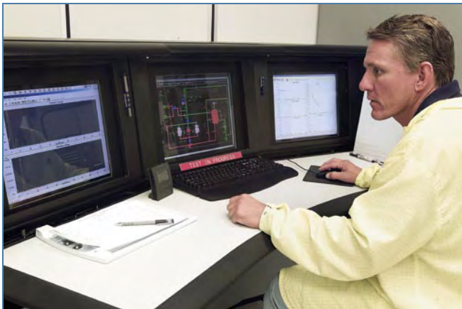
Managing the tritium loading process through the data acquisition and control station interface.
