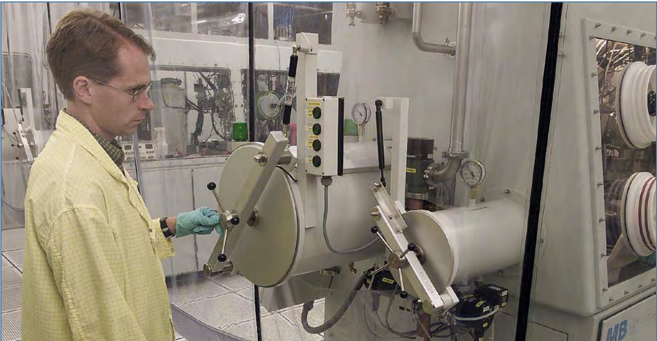
Activating the evacuation/purge cycle prior to glovebox pass box operations. (A pass box provides a way to safely insert material into a glovebox or remove material from it.)
