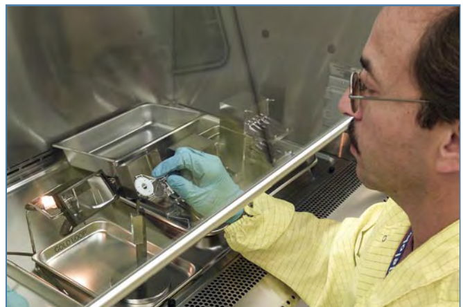
Manipulating an incoming WR target in preparation for the tritium loading process.
